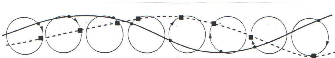
Figure 1. The orbits of surface particles in a deep water wave. The particles move from ● to ■ as the wave moves from the full curve to the broken curve.
